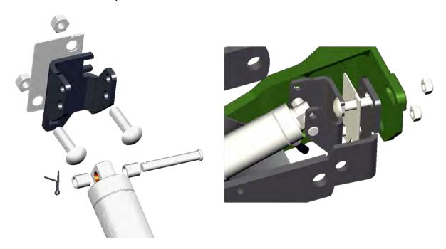
Tighten to 75 lb-ft of torque.
