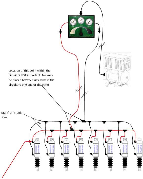
Note: the Lift Circuit line must be connected to the port towards the row cleaners (or rod portion of the cylinder)
