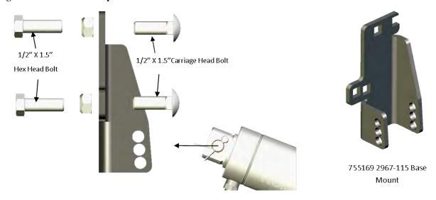
Install the base of the Cylinder to this bracket using the Cylinder Base Pivot Pin (755018). Use the two -5/8" OD X 7/16ID X 0.688"L Spacer Bushings to properly secure and align the cylinder in the Base Mount Bracket
