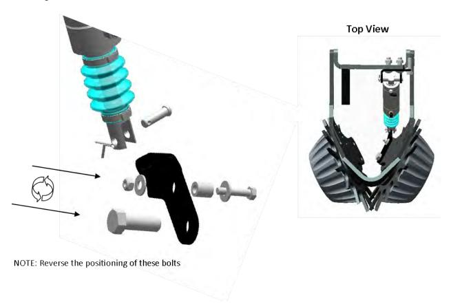
This will require removal of the existing 5/8" Bolt installed through the hub. When re-installing, re-use the existing 5/8" washer, ensure proper alignment of all components, and that the hub is firmly secured.
