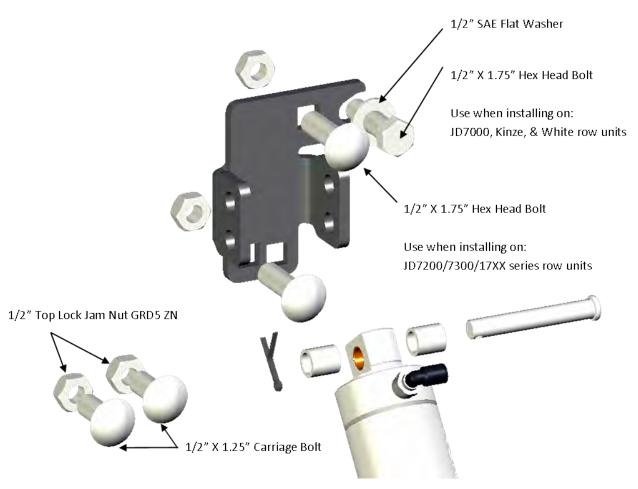
Install the base of the Cylinder to this bracket using the Cylinder Base Pivot Pin (755018). Use the two - 5/8" OD X 7/16ID X 0.688"L Spacer Bushings to properly secure and align the cylinder in the Base Mount Bracket.
