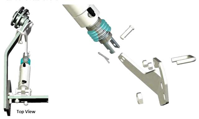
Secure the Rod Mounting Bracket to the clevis yoke on the cylinder using the supplied cylinder rod pivot pin (755019) and cotter pin. Refer to the Mounting Hole Selection guide at the end of this section for more information on which mounting holes to use with this bracket.
