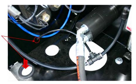
It is intended that the supplied brown colored tubings is used from the compressor to the control box to help color code the line as the air supply for ease of attachment to the system by the user.
