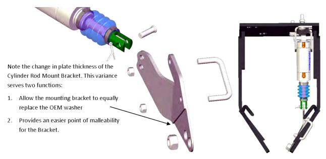
Secure the Rod Mounting Bracket to the clevis yoke on the cylinder using the supplied cylinder rod pivot pin (755019) and cotter pin. Refer to the Mounting Hole Selection guide at the end of this section for more information on which mounting holes to use with this bracket.
