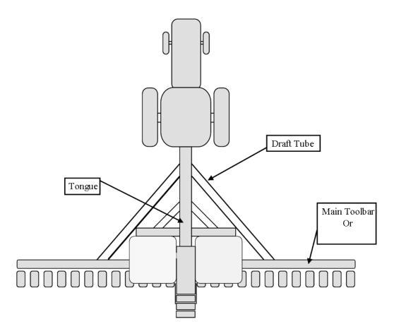
The diagram to the right will help identify possible mounting locations on your specific planter. Allow room for the lid to open properly. Measure 10" vertically and 8" to the rear of the point marked with an \*. The 'X' dimension is the spacing between the tank rail bolt holes, on center. The bolt holes are spaced 1" on center, with 1" slots at each end.
