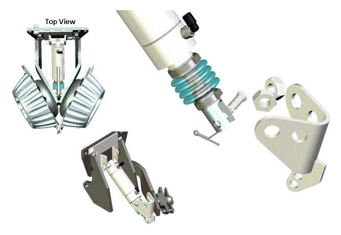
When installing the Cylinder Rod Mount Bracket, be sure it is properly aligned in the clevis yoke of the Rod and firmly seated in the curve of the row cleaner. This may require the exact angle of the bracket to be tweaked or modified in order to more perfectly match the individual row unit.
