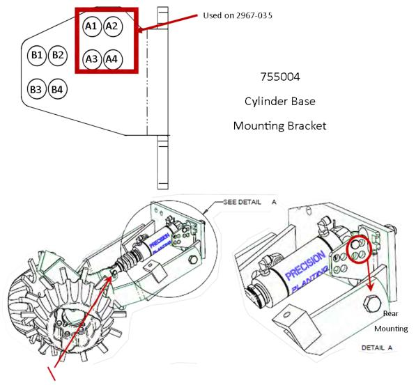
The hole used on the Rod Mount Bracket should correspond to the same hole used on the Base Mount Bracket. Example: Top to Top and Bottom to Bottom
