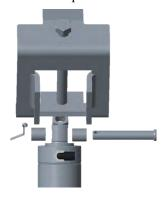
Secure the base brackets to the face place with the 1/2" x 6" bolt and the 1/2" hex nut.
