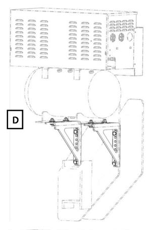
This mounting kit will be very similar to the previous mounting kit. The same brackets will be provided, however there will also be two U-bolts, removing the need for a drilling operation.
