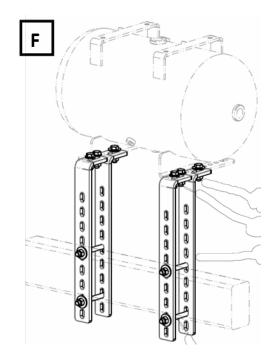
This mounting kit is designed for situations that do not allow mounting on the planter, or require greater elevation of the compressor for clearance reasons. Two of the brackets (shown below right), two straps, two U-Bolts, and hardware will be supplied. The image at left shows the compressor mounted above the 2 point cross-hitch
