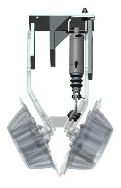
When installing the Cylinder Rod Mount Bracket, be sure it is properly aligned in the clevis yoke of the Rod. This may require the exact angle of the bracket to be tweaked or modified in order to more perfectly match the individual row unit.
