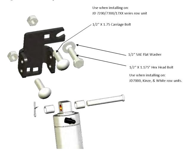
Install the base of the Cylinder to this bracket using the Cylinder Base Pivot Pin (755018). Use the 5/8" OD X 7/16ID X 0.688"L Spacer Bushing (towards the interior of the row) and the 5/8" OD X 7/16ID X 0.829"L Spacer Bushing (towards the exterior of the row) to properly secure and align the cylinder in the Base Mount Bracket.
