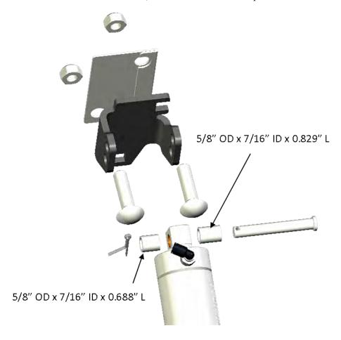
Install the base of the Cylinder to this bracket using the Cylinder Base Pivot Pin (755018). Use the 5/8" OD X 7/16ID X 0.688"L Spacer Bushing (towards the interior of the row) and the 5/8" OD X 7/16ID X 0.829"L Spacer Bushing (towards the exterior of the row) to properly secure and align the cylinder in the Base Mount Bracket.
