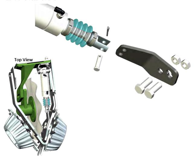
Secure the Rod Mounting Bracket to the clevis yoke on the cylinder using the supplied cylinder rod pivot pin (755019) and cotter pin. Refer to the Mounting Hole Selection guide at the end of this section for more information on which mounting holes to use with this bracket.
