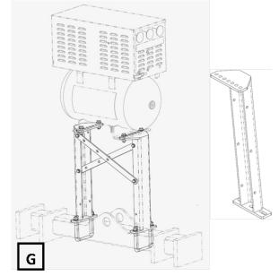
This mounting kit will locate the Compressor low and to the side of the main tongue. Used primarily for Kinze planters to provide clearance under the Lift and Twist transport. Two brackets, two U-bolts, and hardware will be supplied with this kit.
