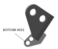
**Note:** In general, all rows will be set to the same hole. However, some rows may require unique settings. A typical example would be a row unit directly behind a tractor tire. In this example, this row unit should be set to exert more force on the row cleaner than the surrounding rows. If the system is normally operated in LIFT mode, install this row unit in the <u>bottom</u> hole. If the system is normally operated in the DOWN mode, install this row unit in the <u>top</u> hole.
