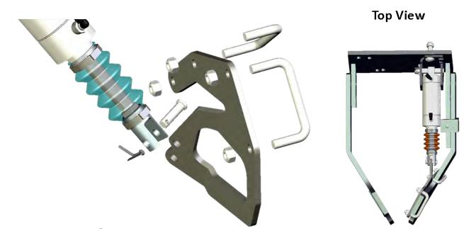
Secure the Rod Mounting Bracket to the clevis yoke on the cylinder using the supplied cylinder rod pivot pin (755019) and cotter pin.
