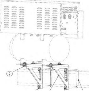
The most common mounting location for larger planters will be on the draft bar. Use this mounting kit for situations that do not provide enough clearance for the compressor to rest directly on the draft bar. Four of the straps shown at left as well as hardware will be provided. This will allow the compressor to be elevated and set back (or forward) to avoid clearance issue.
