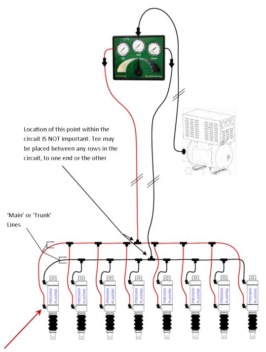
Note: the Lift Circuit line must be connected to the port towards the row cleaners (or rod portion of the cylinder)
