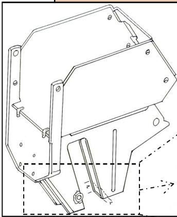
Owners of White 5100 planters will need to make a frame modification to accommodate the Firmer. After removing the gauge wheel and disk opener, you must remove a portion of the row unit's shank frame.
