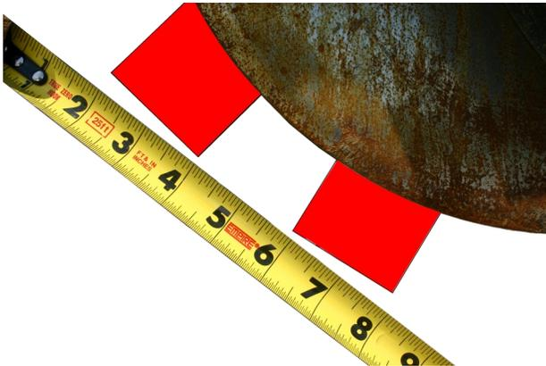
**Correct Contact Between Disk Openers**
