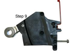
(Step) Next, run the zip tie provided through the 7/32" hole in the Universal bracket and route the zip tie around the metal stiffener bracket. Position the zip tie so the knot is toward the back and inside of the stiffener bracket. Cut off excess length of Ziptie.
