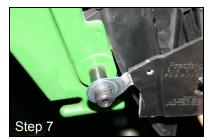
Place the lower end of the XP Rear Mount Stiffening bracket inside the rounded notch.
