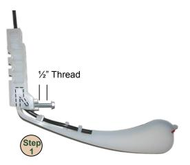
First, route the tube through the hose channel. Make sure the tubes are clear of the tension screw. Assemble 2-piece liquid firmer by inserting the Tail into the Poly Mounting Bracket as shown above. Make sure tension screw is below the tab on Tail section.
