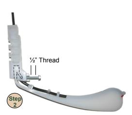
Lower the drill so the opening disks rest on a flat surface or on the floor. Remove the outside disk opener from the row unit.
