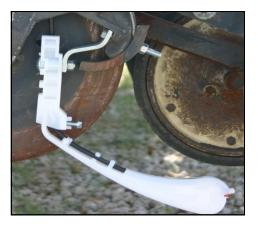
Next, locate the disk scraper mounting hole on the casting. Bolt the Firmer mounting strap to the casting using the 3/8" X 3" bolt. Tighten with lock washer and nut.
