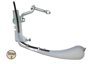
Bolt the Steel Bracket (with the hole furthest away from the edge) to the top hole of the firmer using 3/8" X 2" the carriage bolt provided. The head of the bolt should seat into the slot on the front side of the Firmer. Tighten with lock washer and nut.
