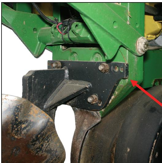
Note: Stops are not needed if row mounted coulters or row cleaners already create a stop by extending their mounting bracket out between the face plate and parallel arm stop.
