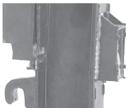
Offset Sensor to Reduce Seed Catchpoints
