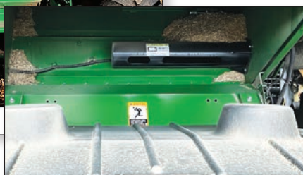
A tailboard, with the Tailboard Trash Blower Tube, after a full season of harvesting soybeans.
