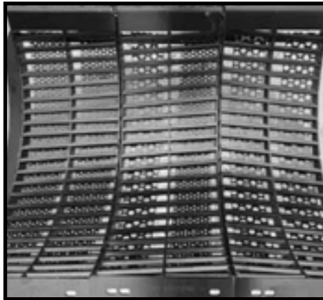
Angled bars, in different directions, improve thrashing
