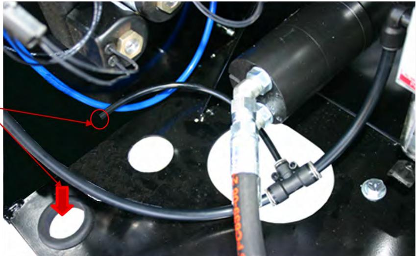
It is intended that the supplied brown colored tubings is used from the compressor to the control box to help color code the line as the air supply for ease of attachment to the system by the user.
