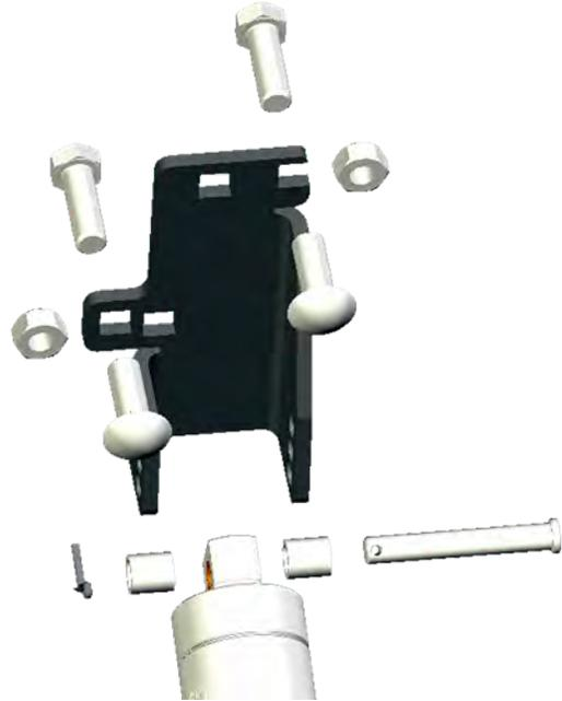
**Tighten to 75 lb-ft of torque.**
