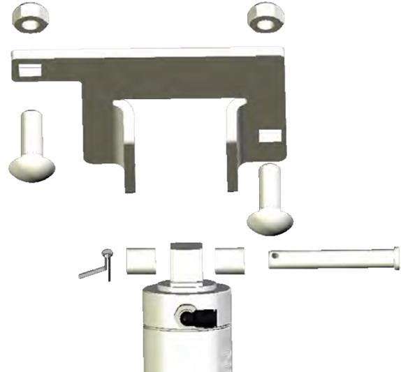
**Tighten to 75 lb-ft of torque.**
