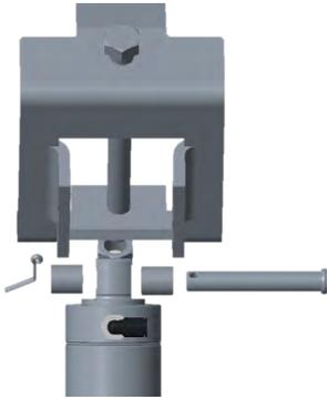
**Tighten to 75 lb-ft of torque.**
