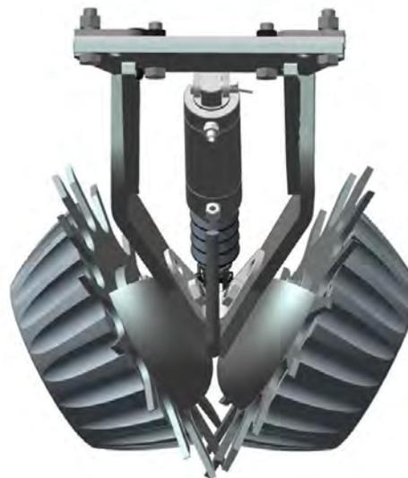
When installing the Cylinder Rod Mount Bracket, be sure it is properly aligned in the clevis yoke of the Rod. This may require the exact angle of the bracket to be tweaked or modified in order to more perfectly match the individual row unit.
