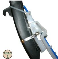
Next place the stainless steel clamp around the seed tube and the Firmer. Make sure the clamp is at the bottom of the notch and its head is centered under the Firmer so it cannot rub on the rolling opening disc. Tighten the clamp snugly and trim off the excess.
