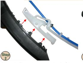
Place the Firmer base on the back of the seed tube and slide the Firmer up until the lip on the base of the Firmer is next to the opening of the seed tube. The base of the Firmer should cover the bottom two fins on the tube. Slide a tie through the hole at the top of the Firmer and secure it around the seed tube above the tube's hook.
