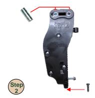
Cut the zip ties that hold the brackets together for shipping. Secure the two pieces of each bracket together with four 10-24 x 1" carriage bolts and locking nuts and one 1" machine screw. Install the pipe spacers into the bracket.
