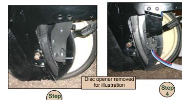
Slide the bracket assembly up inside the row unit frame. Align the top two holes of the bracket with the inside of the scraper bracket holes on the planter frame.
