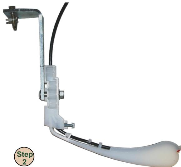
Using the second to the top round hole of the firmer, bolt the firmer to the back of the mounting bracket with 3/8" bolt, washer, and hex nut provided.
