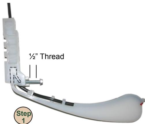
First, route the tube through the hose channel. Make sure the tubes are clear of the tension screw. Assemble 2-piece liquid firmer by inserting the Tail into the Poly Mounting Bracket as shown above. Make sure tension screw is below the tab on Tail section. Then tighten the tension screw leaving a 1/2" of thread showing between the bracket and the head of the tension screw.
