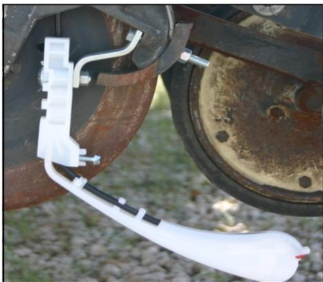
Next, locate the disk scraper mounting hole on the casting. Bolt the Firmer mounting strap to the casting using the 3/8" X 3" bolt. Tighten with lock washer and nut.
