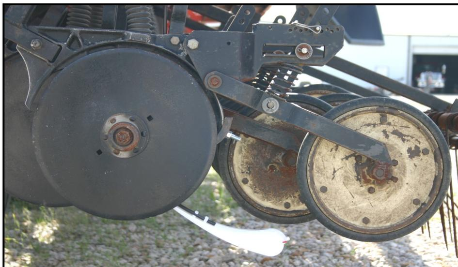
**Backing Up** tractor while drill is not fully raised can result in damage to the Keeton Seed Firmers.
