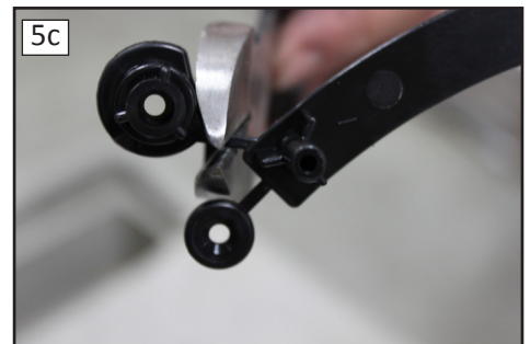
Clip the washer from the Singulator shim molding.
